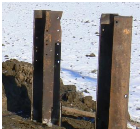
Figure 5.8. Local buckling and bending damage to two steel anchor piles due to driving
