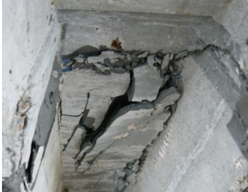
Figure 5.47. Damaged region of UHPC Pile 1 at the end of the lateral load test
