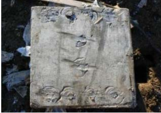
Figure 5.13. Condition of pile head at the end of driving pile P1
