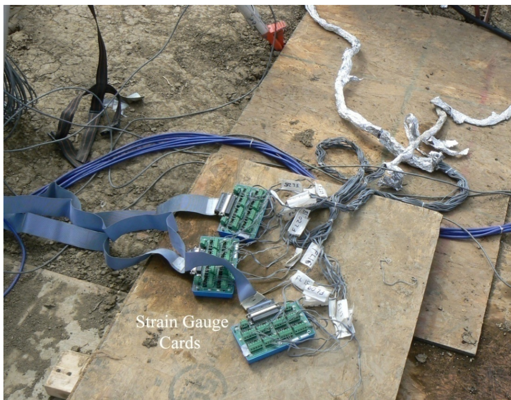
Figure 5.32. Data collection system used during the lateral load test (continued)
