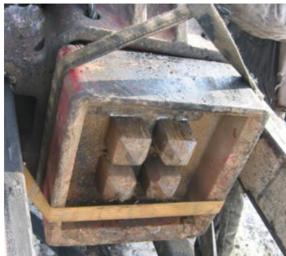
Figure 5.5. Driving helmet with guiding spikes used for steel piles
