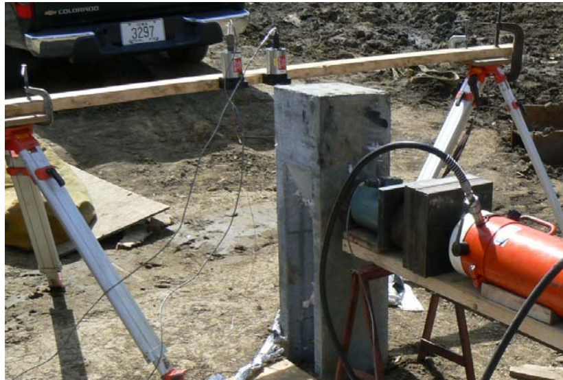
Figure 5.30. Displacement transducers attached to a wooden reference beam, supported on tripods
