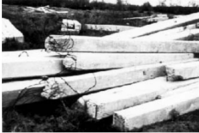
Figure 1.1. Precast, prestressed concrete piles damaged during hard driving (DiMillio 1998)
