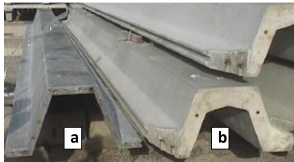
Figure 2.43. Comparison of a) SCFRC and b) conventional concrete sheet piles (Grünewald 2004)
