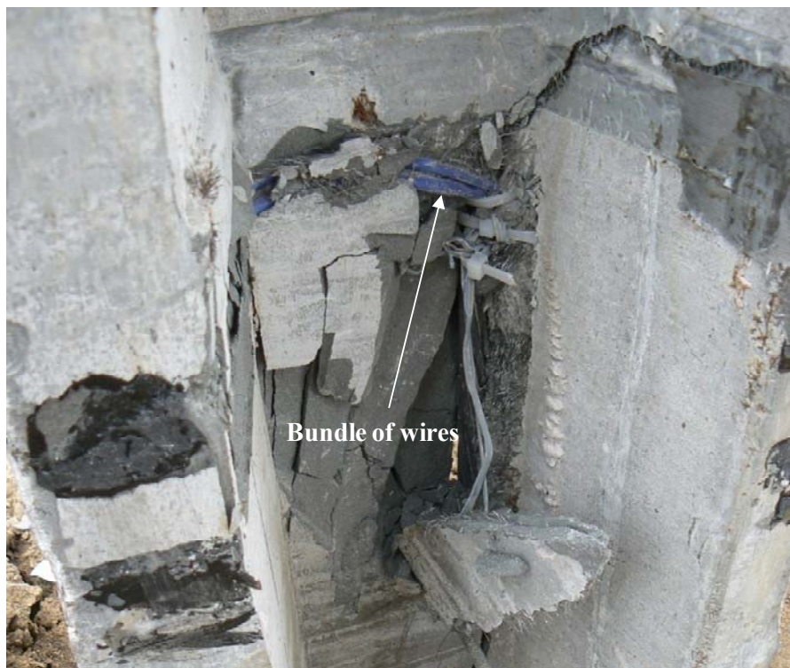
Figure 5.49. Shear failure region of UHPC pile P1 after the lateral load test with some cracked UHPC pieces removed
