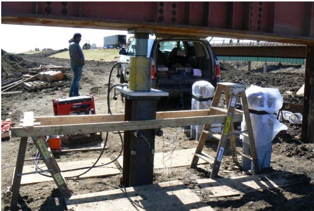
Figure 5.19. Wooden reference beams supported by ladders (steel pile)
