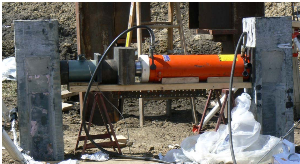
Figure 5.34. View showing the lateral load test set-up at the beginning of the load test
